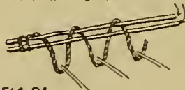
FIG. 94 SOUTHERN NIGERIA IMP. INST. TYPE OF HEDDLE IN USE WITH WEST AFRICAN VERTICAL COTTON LOOMS
